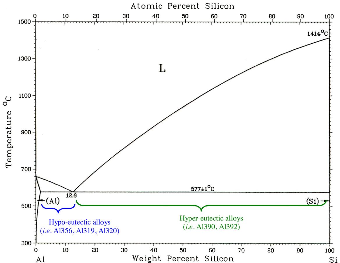
Fig. 1. Al-Si phase diagram showing hypo- and hyper-eutectic alloys.
